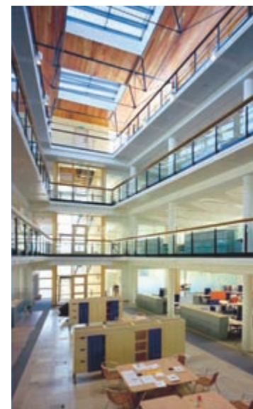
Atrium, showing exposed concrete frame.
